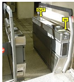
automatic ticket gate
